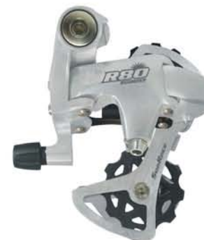
RDR81 SD/LD [Alloy Bracket & Outer Link] [8-Speed]
