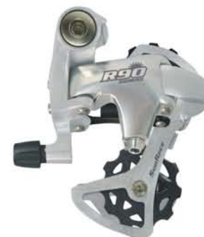
RDR91 SD/LD [Alloy Bracket & Outer Link] [9-Speed]
