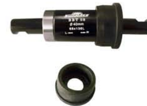
BBT08 5[35mm] 8[38mm] 4[40mm] [Steel Axle] [Eng. Polymer RH & LH Cups] [Steel Sleeve] [Eng. Polymer Stopper] [Sealed Cartridge Bearings]
