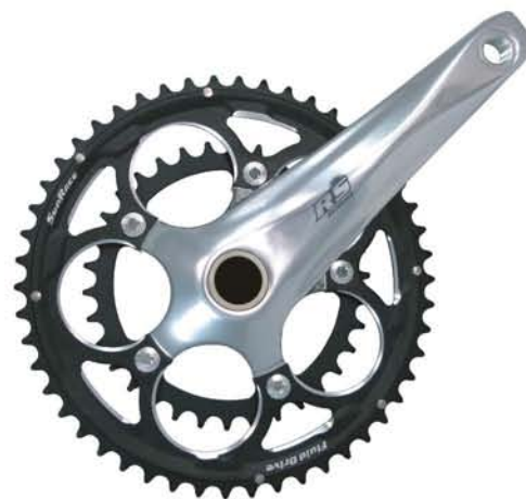
FCRS6 (S1) 50-34T [BCD 110mm] [6061 Forged Alloy Crank] [Alloy Chainrings] [7075 Bolts & Nuts] [7075 Axle Bolt] [944g/949g incl. BB] FCRS1 (S1) 53-39T [BCD 130mm] [6061 Forged Alloy Crank] [Alloy Chainrings] [7075 Bolts & Nuts] [7075 Axle Bolt] [944g/949g incl. BB]
