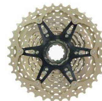
CSMS TAW 11-36T [10-Speed] [2-Piece Alloy Spider] M[Champagne] [348g]
