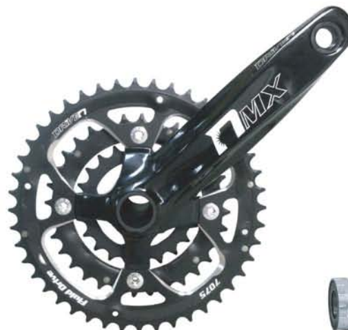
FCMX7 (D1) 44-32-22T [6061 Forged Alloy Crank] [Chromoly Axle] [7075 Chainrings] [7075 Bolts & Nuts] [7075 Axle Bolt] [851g incl. BB]
