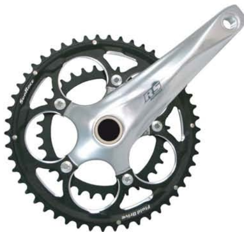
FCRS6 (S1) 50-34T [BCD 110mm] FCRS1 (S1) 53-39T [BCD 130mm] [6061 Forged Alloy Crank] [Alloy Chainrings] [7075 Bolts & Nuts] [7075 Axle Bolt] [944g/949g incl. BB]
