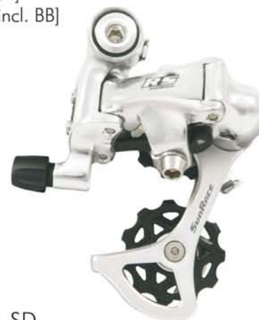
RDRS SD [7075 Bracket Bolt] [Alloy Links] [Alloy Cage] [10 & 9-Speed] [195g]
