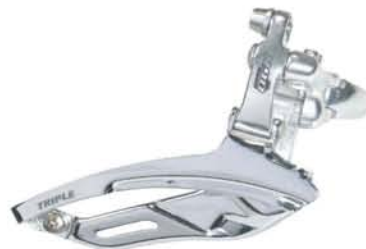
FDR99 BB/LB/MB [50T] [Triple] [Forged Alloy Links]
