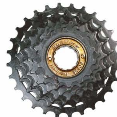
MFM05 7DS 14-28T 6DS 14-28T 5DS 14-28T [Friction]
