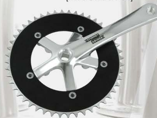
FCT22 42T FCT24 44T FCT26 46T FCT28 48T [6061 Forged Alloy Crank] [Polished Anodized Finish] [PCD 130mm] [7075 Chainring] [SCM435 Bolts & Nuts]
